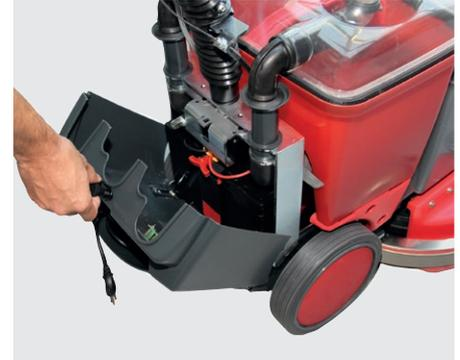
Fast access to battery cause of simple tray
