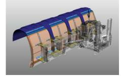
2. an adjustable snow deflector made of cloth. This version is particularly suitable for powder snow and high speeds. A combination with the polyurethane or rubber snow deflector is possible.
